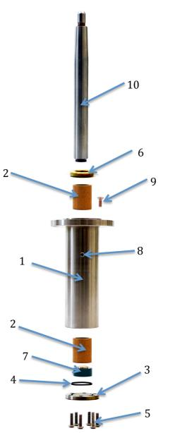
The bearing comes pre lubricated from the factory but before use the felt washer (6) should be loaded with several drops of the oil provided to ensure it is quite moist. It is worth checking periodically that the felt washer has not dried out as this feeds the Oilite bushes (2), keeps them lubricated and prevents them from drying out. The oil will work its way down to the bottom bush and keep it sufficiently "oiled"
